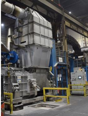
A large industrial furnace, identified as a StrikoWestofen MH II-T model, is shown in a factory setting. The furnace is a tall, cylindrical structure with a metallic exterior and various pipes and structural elements around it. | <b>1,00 €</b> |
