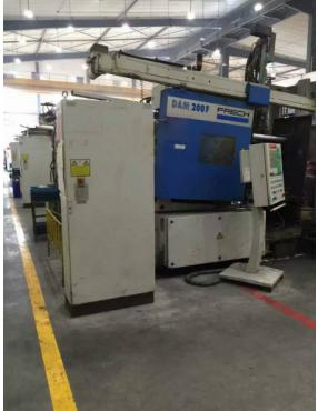
A large industrial Frech DAM 200 F machine, a hot chamber casting machine for magnesium, model WK1440. It is a blue and white machine with a control panel and a robotic arm. | <b>1,00 €</b> |
