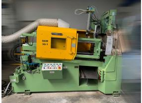
A large industrial casting machine, specifically a Frech DAW 50 model, designed for low-pressure casting with a hot chamber. It has a green base frame and a yellow control cabinet on top. The machine is shown in a workshop environment. | <b>1,00 €</b> |
